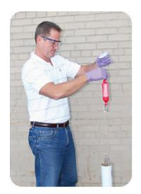
Passive sampling significantly reduces the field costs and time associated with groundwater well monitoring, reduces field sampling variability, can provide vertical profiling of contaminate concentrations, and has no known depth limit. Passive samplers are easy to deploy and retrieve and may be used in conjunction with one another.
