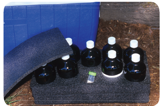
Final layer of thin foam atop the samples
