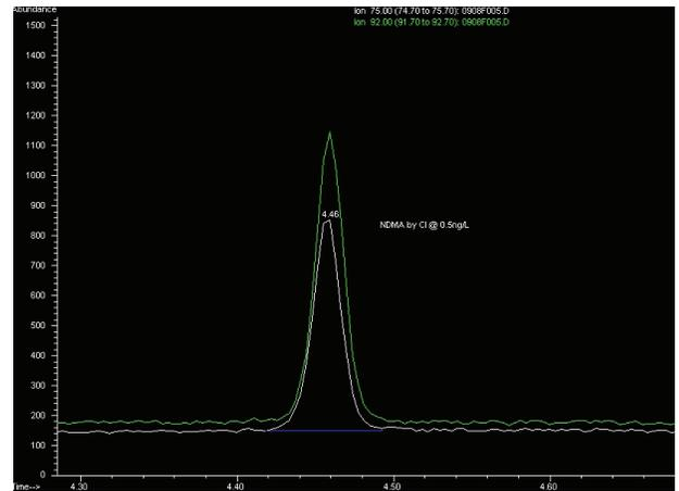
Figure 1b. EICs of NDMA of a 0.5ng/ml calibration standard
