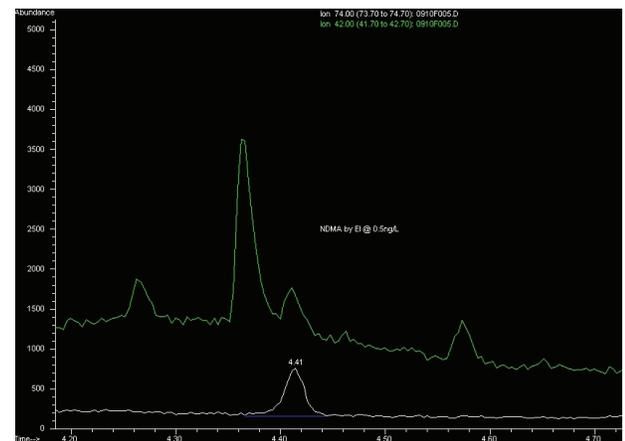
Figure 2. Total Ion Chromatograms of 1.0ng/L NDMA in a Lab Fortified Sample
